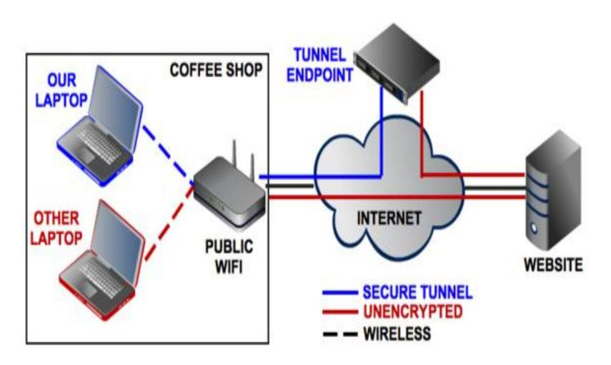
This diagram illustrates the difference between using an unencrypted connection and using a VPN-secured Internet connection at your average coffee shop.
